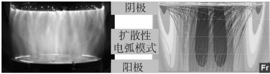
图7 40 kA 电流开断与等离子体流和磁收缩力模拟图 Fig. 7 Verification of AMF arc model of 40 kA arc and simulated plasma flow and magnetic constriction forces
